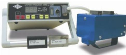
obtain another diagram of loading, stress vs. coercivity or deformation vs. coercivity. Coercivity here may increase from an initial value of the metal (as-delivered condition), on the way to its failure, 2 ÷ 4 times (!), depending on the brand of metal. In this test, the specimen is subject to planar uniaxial stress loading. This is the simplest version of simulation of actual fatigue process that occurs in
